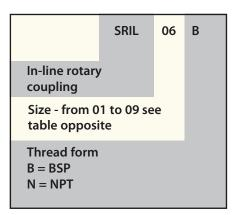
Example: SRIL 06 B Rotary Coupling, 1 1/4" BSP ports.
